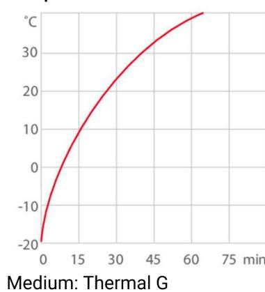
**Temps de refroidissement**
